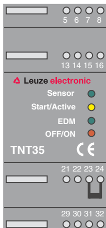
Figure 4.2-11: Operating mode "without start- and restart-disable"
