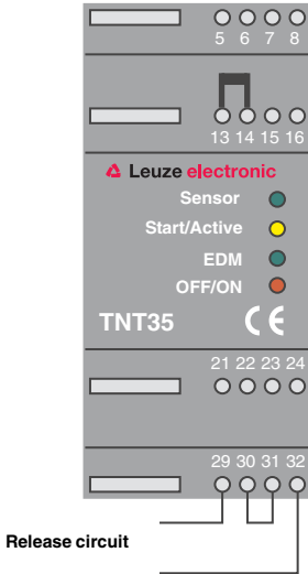
Figure 4.2-6: Wiring safety output (one-channel release circuit)
