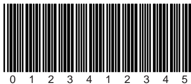
Figure 8.2: Bar code sample (Code 39; 0.35 mm; print ratio 2:1)
