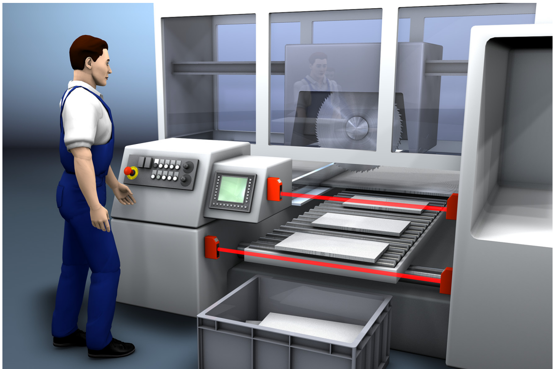
Figure 5.2: Access guarding / intervention control on sawing machines
