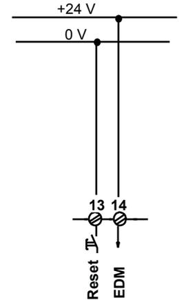
In this case, the start/restart interlock function and the dynamic monitoring of the downstream relays, which may be required in order to maintain the safety category, must be performed by other means.
