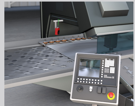
Rear area monitoring in punching machine
