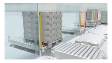
Space saving: Smart Process Gating does not require any additional trigger sensors for bridging of the protective function, thereby allowing a particularly compact system design.
