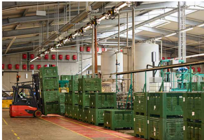
In the transfer area, it is essential that processes are safe – people must not be able to enter the danger zone unnoticed. Access guarding solutions from Leuze are installed above the stations.
