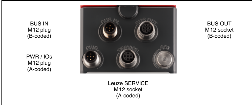
Figure 7.1: Connections of the AMS 3004 i
