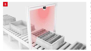
**Solution:** A ROD 300 series laser scanner is mounted above the conveyor system. The frequency of the individual scans of the ROD 300 can be increased so that the blind areas between two measurements are minimized and the objects can be detected even faster. This maximizes production throughput and system efficiency.
