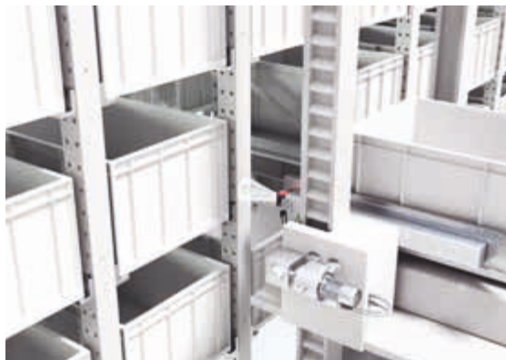
IPS 200i: Fine positioning on column in the container warehouse
