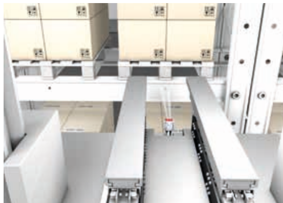
IPS 400i: Fine positioning on bar in double-depth pallet warehouse
