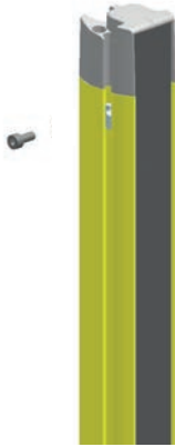
Fig. 5.7: Mounting via sliding blocks
