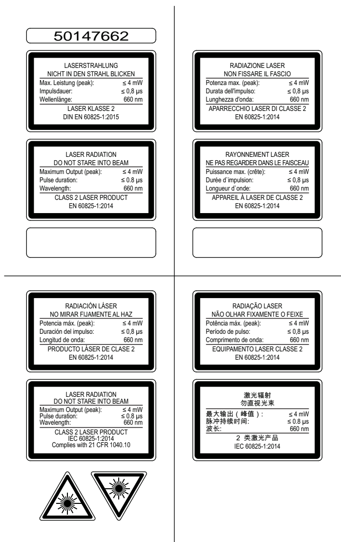
Fig. 2.2: Laser warning and information signs – supplied stick-on labels
