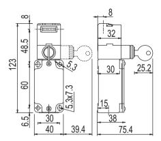
Figure 3.5: Dimensions of L10-M3C1-M20-KO in mm
