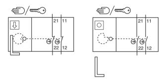
Figure 7.1: Contact block 2NC (L10-P2C1-M20-SB20, L10-M2C1-M20-SB20)
