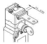
Secure actuator with rivets or tamperproof screws so that it cannot be detached.
