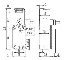
Figure 3.1: Dimensions of L10-P2C1-M20-SB20 and L10-P3C1-M20-SB20 in mm
