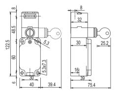
Figure 3.4: Dimensions of L10-P3C1-M20-KO in mm
