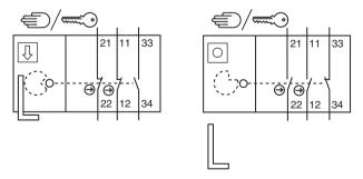
Figure 7.2: Contact block 2NC + 1NO (L10-P3xxx, L10-M3xxx)
