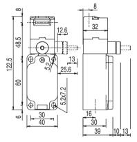
Figure 3.2: Dimensions of L10-M2C1-M20-SB20 and L10-M3C1-M20-SB20 in mm
