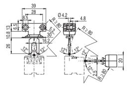
Figure 13.6: AC-AH-F4J2-TK actuator
