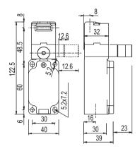
Figure 3.3: Dimensions of L10-P3C1-M20-LB10 and L10-P3C1-M20-LB20 in mm
