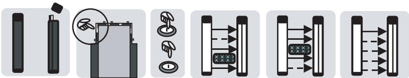
**Fig. 4.3-8:** Turning on reduced resolution with the switches S4/S5, example with start/restart interlock
