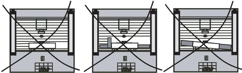
Fig. 4.3-2: Shadows in the protective field must always be prevented.
