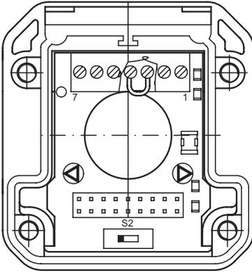
**Fig. 7.2-1:** Transmitter connection cap/T1 removed, terminal field inside view
