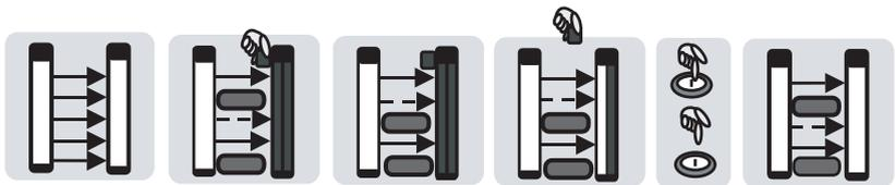
**Fig. 4.3-6:** Simultaneous teaching-in of a fixed and (after selection with S4/S5) a floating blanking zone
