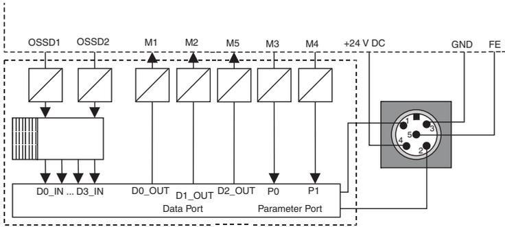
**Fig. 7.9-5:** Machine interface /A1, schematic structure
