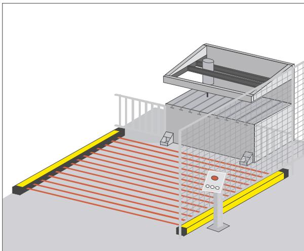
**Fig. 3.4-2:** COMPACT*plus-b* Safety Light Curtain – Application for a routing machine
