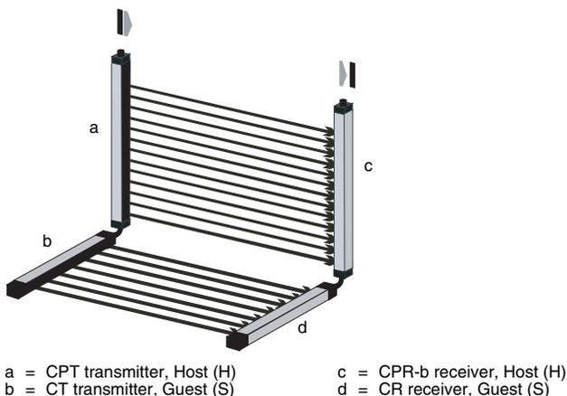
**Fig. 3.2-1:** Structure of a cascaded system
