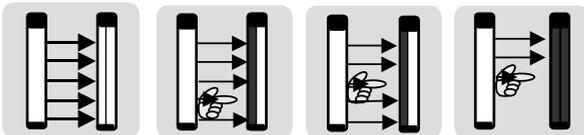
Fig. 3.1-2: Example: MultiScan, scan-related, MultiScan factor H = 3
