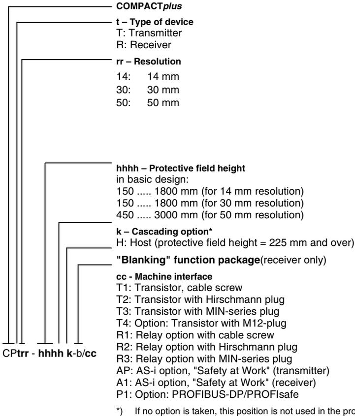
Fig. 1.3-1: Selecting COMPACTplus-b Safety Light Curtains
