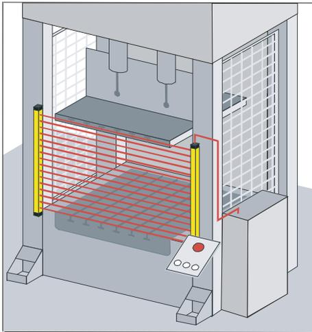
**Fig. 3.4-1:** COMPACT*plus-b* Safety Light Curtain – Application for a press
