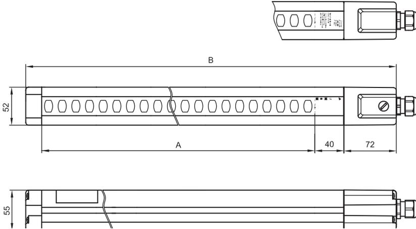
**Fig. 12.2-1:** Dimensions Safety Light Curtains
