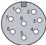
**Fig. 7.1-1:** Receiver – local connection socket, M12, 8-pin
