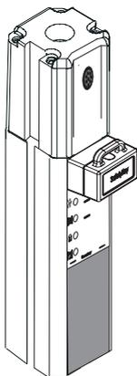
**Abb. 9.2-1:** Setting the SafetyKey on a light curtain's receiver
