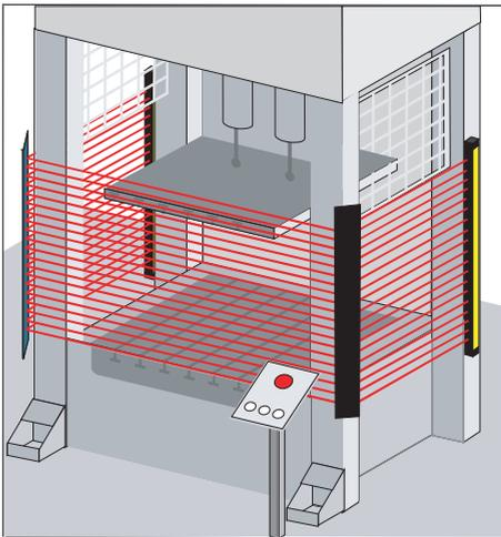
**Fig. 3.3-1:** Example: Multiple-side protection of a danger point using deflection mirrors.
