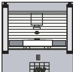
**Fig. 4.3-1:** Mechanical locks of equal sizes must prevent entry into the protective field from the side with fixed or floating objects.
