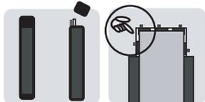
**Fig. 4.3-5:** Switching on the teaching-in option for floating blanking with S4/S5
