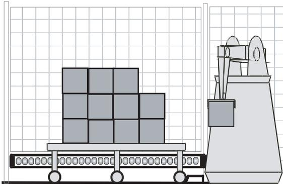
**Fig. 4.3-9:** Example: Reduced resolution permits beam interruptions of defined sizes.
