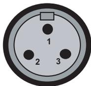
Fig. 7.4-1: Transmitter interface /T3, MIN-series plug, 3-pin – view of the plug pins
