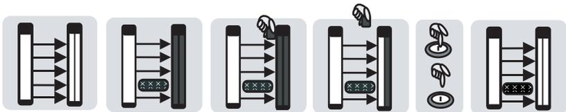
Fig. 4.3-3: Teaching-in of fixed blanking zones with the SafetyKey
