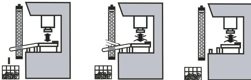
**Fig. 4.3-4:** Example of "Fixed blanking"
