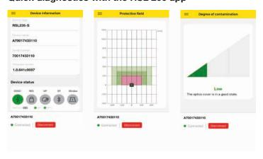
The RSL 200 app enables easy access to status information and diagnostic data via Bluetooth - even if the RSL 200 is installed in areas that are difficult to see or access to the device is restricted. Bluetooth remote access does not affect machine availability. is not impaired. All messages are displayed in plain text and can also be sent directly to Leuze Service if required.
