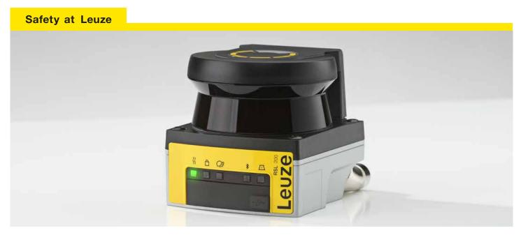
With their dimensions of 80 x 80 x 86 mm, the compact RSL 200 safety laser scanners take up very little space and and can therefore be easily and unobtrusively integrated into the machine design. With a range of 3.00 m and a 275° scanning angle, they offer cost-effective solutions for many standard area guarding tasks.
