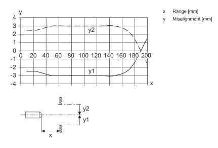
Typ. response behavior at 90% diffuse reflection (focusing distance 400 mm)
