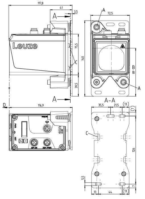
A Adjustment screws with hexagon socket WAF4
