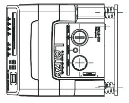
A Center axis of transmitter and alignment laser
