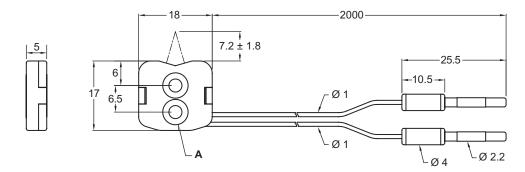
A 2 x Ø 3.2 / Ø 6.2 (mounting hole, on face)
