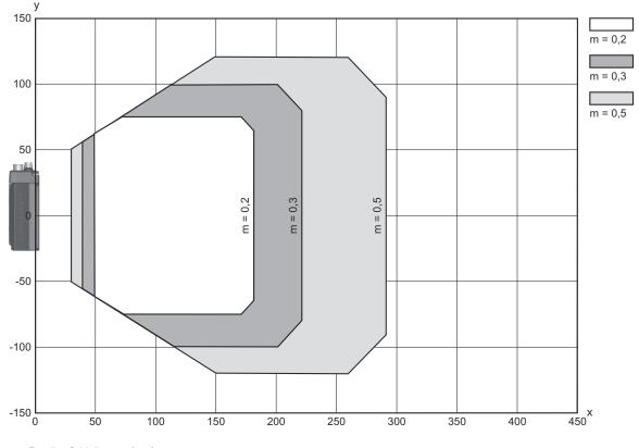
Х Reading field distance [mm]
