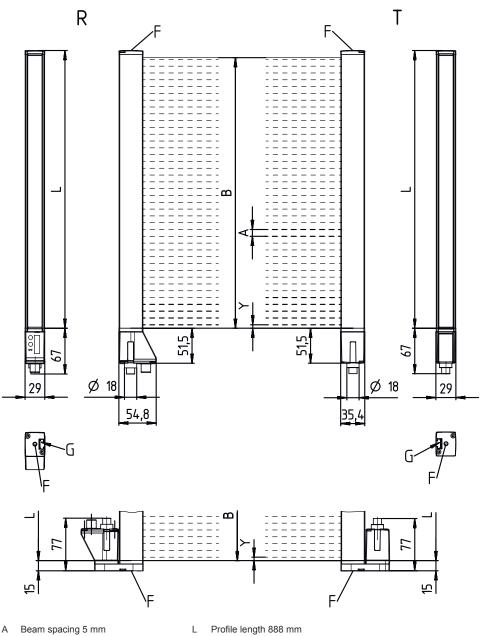
A Beam spacing 5 mmB Measurement field length 880 mm
