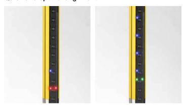
The multi-level alignment display makes commissioning the devices especially easy. Even rough alignments are reliably displayed. Thanks to the well-visible, bright LEDs, the alignment result can be monitored right from the transmitter. The optimal setup is thus quickly achieved. This saves time and money during commissioning and offers reserves in operation.
