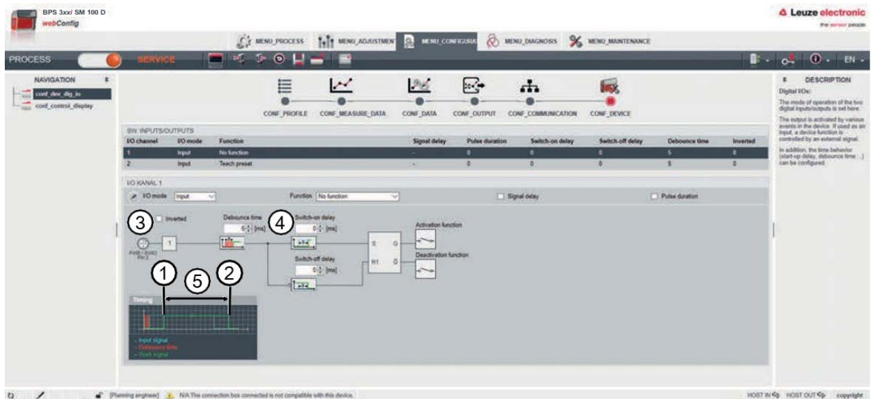
Fig. 10.5: Switch-on delay > 0 and switch-on time > 0
