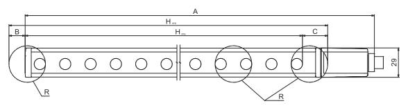
$H_{\text{PFE}}$  Effective protective field height = 1078 mm  $H_{\text{PFN}}$  Nominal protective field height = 1050 mm
