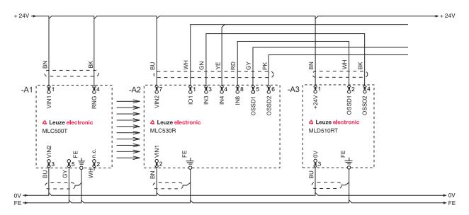
Operating mode 3: circuit diagram example of a linked, contact-based position switch for monitoring of the blanked object and a changeover switch for switching between function groups FG1 and FG2
