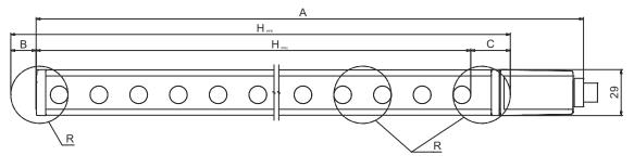
$H_{\mathsf{PFE}}$  Effective protective field height = 1212 mm H<sub>PFN</sub> Nominal protective field height = 1200 mm
