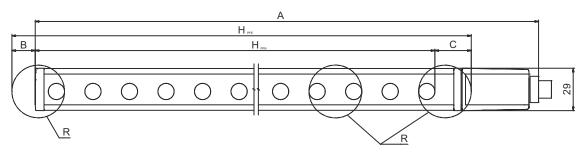
$H_{\text{PFE}}$  Effective protective field height = 1067 mm H<sub>PFN</sub> Nominal protective field height = 1050 mm
