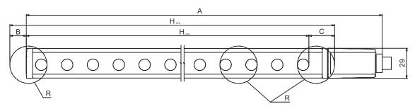
$H_{\mathrm{PFE}}$  Effective protective field height = 1540 mm H<sub>PFN</sub> Nominal protective field height = 1500 mm
