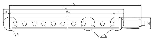
$H_{\mathsf{PFE}}$  Effective protective field height = 940 mm H<sub>PFN</sub> Nominal protective field height = 900 mm
