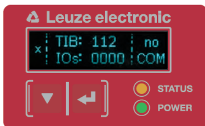
Figure 3.6: Function buttons on the receiver
