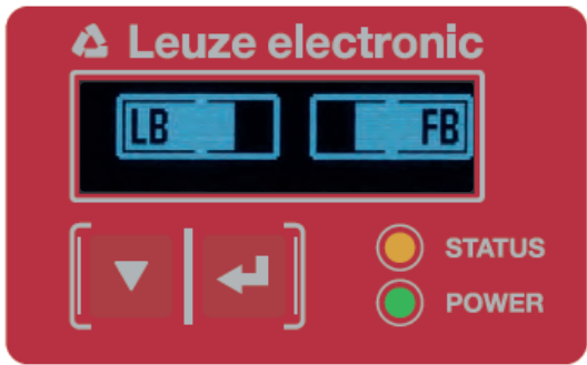
Figure 8.7: Display after successful teach The next configuration step is to check the alignment.
