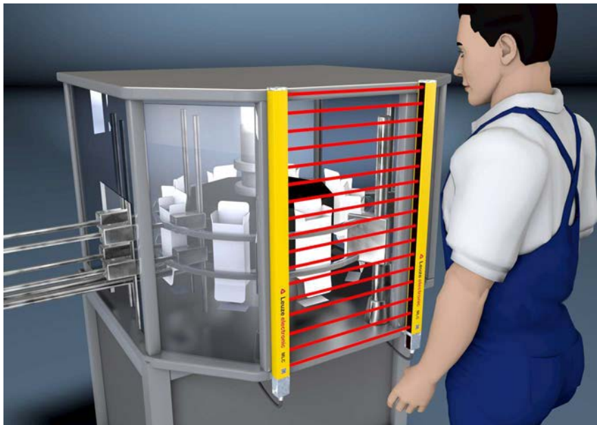
Fig. 5.1: Point of operation guarding protects reaching into the danger zone, e.g. for cartoners or filling systems
