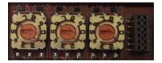
The default setting is 000 as shown above. The arrow points to the switch location. 0 is located at the 3:00
