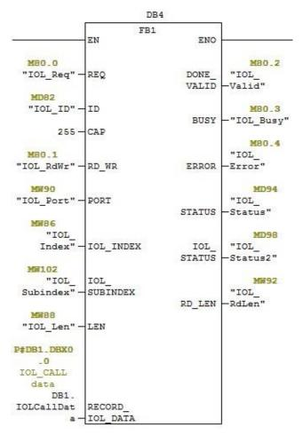
Figure 56: IOL\_CALL Function Block
