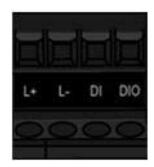
You can connect a digital input device to DI and/or DIO. DIO supports digital out.
