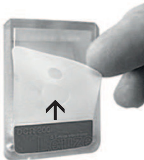
Fig. 6.29: Attaching the diffuser foil
