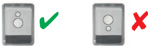
Fig. 6.28: Orientation of the diffuser foil
