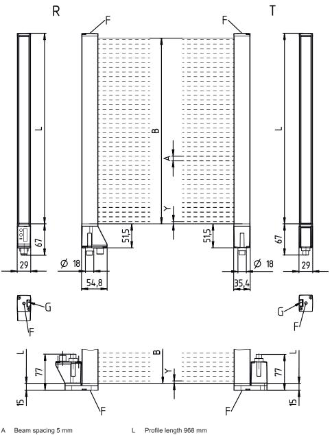
A Beam spacing 5 mmB Measurement field length 960 mm
