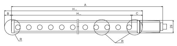
$H_{\mathsf{PFE}}$  Effective protective field height = 540 mm H<sub>PFN</sub> Nominal protective field height = 450 mm
