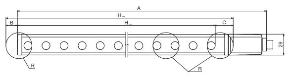
$H_{\text{PFE}}$  Effective protective field height = 1240 mm  $H_{\text{PFN}}$  Nominal protective field height = 1200 mm
