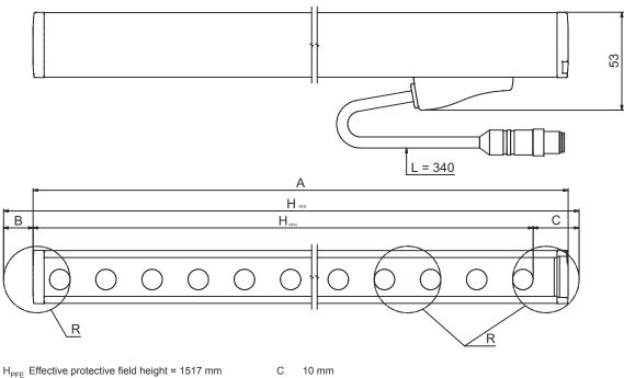
$H_{PFE}$  Effective protective field height = 1517 mm  $H_{PFN}$  Nominal protective field height = 1500 mm
