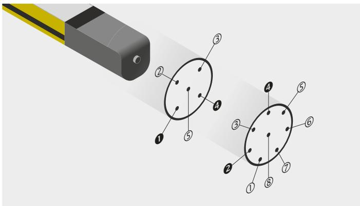
All settings on the device can be configured by means of pin assignment. This saves time and money when commissioning and ensures error-free configuration. A device can be swapped out easily by means of plug&play without reconfiguration.
