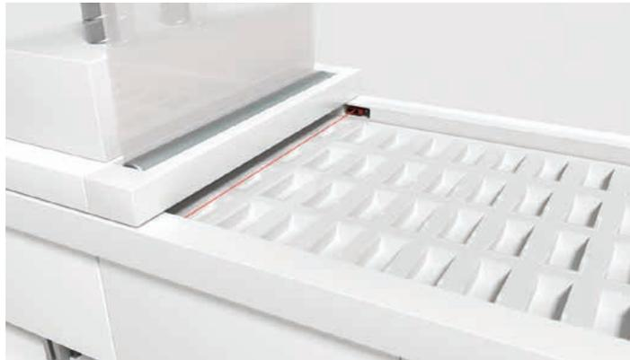
**Solution:** The SLS 46C single light beam safety devices are used at narrow openings. They are available as type 2 and type 4 variants and can be integrated easily via connector or cable.
