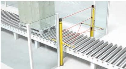
2-sensor muting, time-controlled. Universal solution for entry and exit. The muting sensors are arranged in a cross formation.
