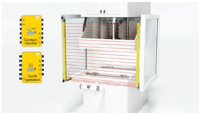
**Solution:** Especially well suited for use on eccentric and hydraulic presses the configuration tool MSI.designer offers a special function library. This contains tailored function blocks for the control and safeguarding of presses, and therefore make quick and easy configuration of the MSI 400 safety control possible.
