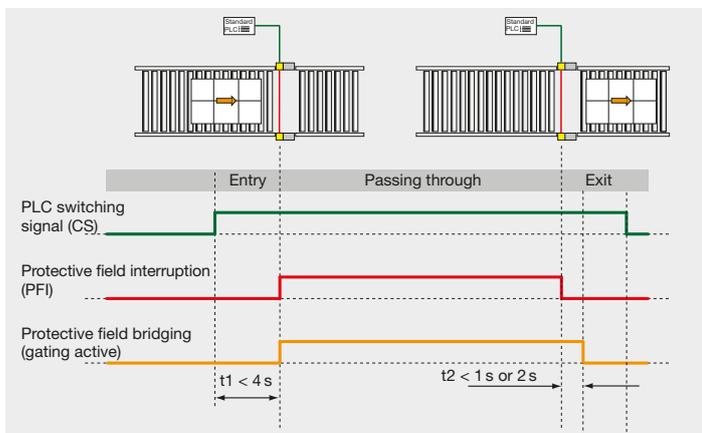
The gating function (bridging of the protective field) is activated by the correct sequence of switching signal and protective field violation and monitored by the light curtain. The gating ends either automatically or – in the case of higher conveyor line speeds – by resetting of the switching signal.
