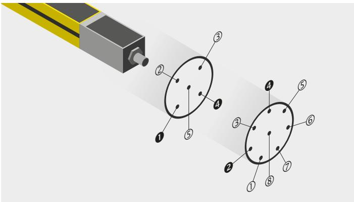
All settings on the device can be configured by means of pin assignment. This saves time and money when commissioning and ensures error-free configuration.
