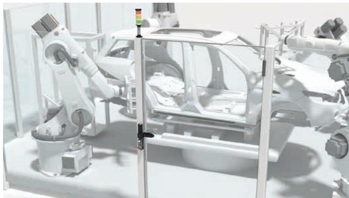
**Solution:** The robust L series safety switches with guard locking keep safety doors securely locked until access is released by an electric signal. The series includes standard designs, devices with integrated operational controls as well as devices with RFID-coded actuators.
