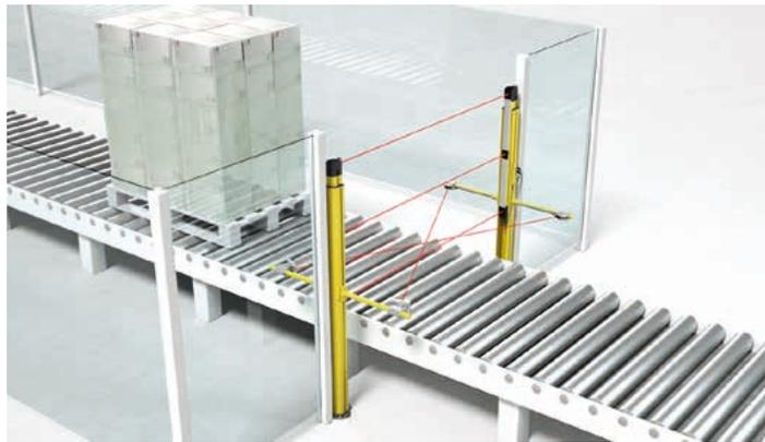
**Solution:** The muting function bridges the safety sensor in a controlled manner to allow the transported goods to pass through. This function is already integrated in the MLD 300/500 multiple light beam safety devices and the MLC 500 safety light curtains. The MSI-MD-FB muting interface and MSI 400 safety control provide an external muting control.
