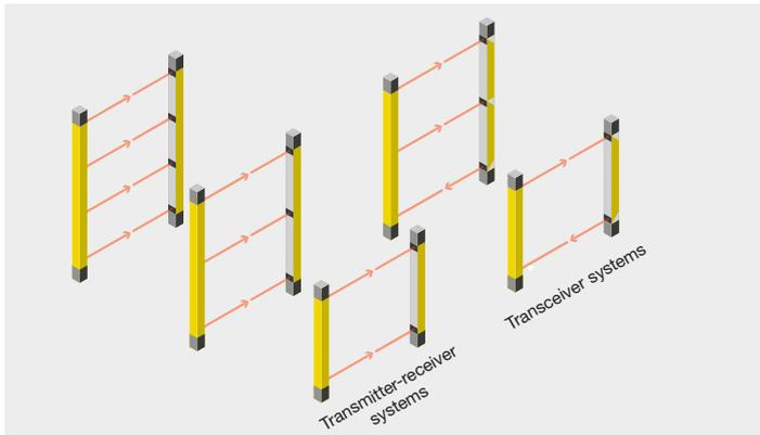
The transceiver systems consist of an active transmitter/receiver and a passive deflecting mirror without electrical connection. This allows cost-effective solutions with low installation effort. The transmitter-receiver systems consist of a separate transmitter and receiver for applications with large operating ranges up to 70 meters. Deflecting mirrors can be added for multi-sided safeguarding.
