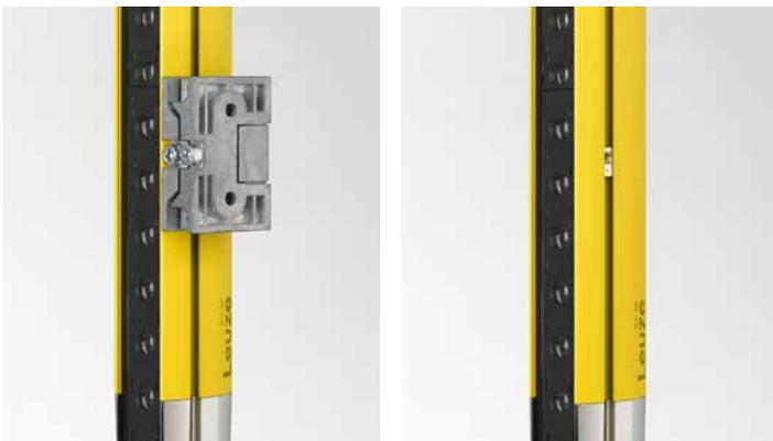
The swivel function of the robust supports facilitate the quick alignment of the devices. These are mounted right in the grooves provided on both sides of the ELC 100. If no alignment is necessary, such as for applications with short operating ranges, the sliding blocks included in the scope of delivery are used, which reduces costs even further.
