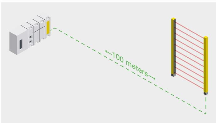
Transmitters and receivers of the MLC 300/500 family can be connected to the switch cabinet using cables measuring up to 100 meters in length.
