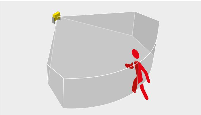
The LBK safety radar sensors detect movements and are used for guarding hazardous areas. They monitor the protected area for access by and the presence of persons. Even persons who are standing still are not really “static”, and are therefore detected reliably by the sensor.
