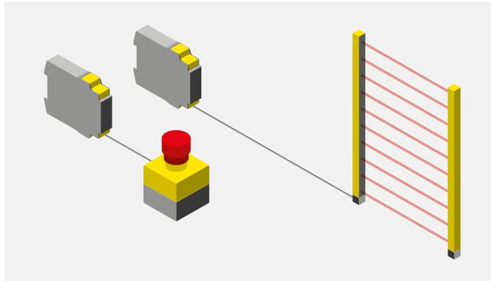
**Solution:** With the reliable MSI safety relays, individual safety sensors can be integrated quickly and easily into the safety circuit of machines and systems. Depending on the model, the relays are tailored to specific applications or can be used universally.
