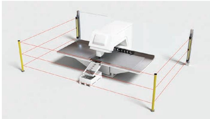
**Solution:** The MLD 300/500 multiple light beam safety devices in combination with the UMC mirror columns safeguard access to the machine on multiple sides and over lengths of up to 70 m. The integrated laser alignment aid makes installation quick and easy.
