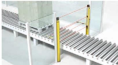
2-sensor muting, sequence controlled. Only for exit zones. For increased requirements, e.g. in terms of shape and position of the load. The muting sensors are aligned parallel to each other.
