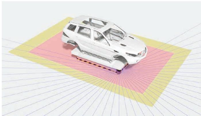
**Solution:** The RSL 400 safety laser scanner merges safety technology and high-quality measurement value output in a single device. It has a scanning range of 270° and 100 reversible field pairs. Two scanners therefore provide optimum guarding of the AGV. The measurement data has a high angular resolution of 0.1° and a low measurement error.
