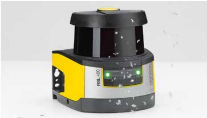
Thanks to the high angular resolution of 0.1°, the RSL 400 is able to filter out non-safety-relevant objects, e.g. dust and particles in the air, particularly well (approx. 3x higher sampling rate than with conventional scanners). This reduces unnecessary switching off.
