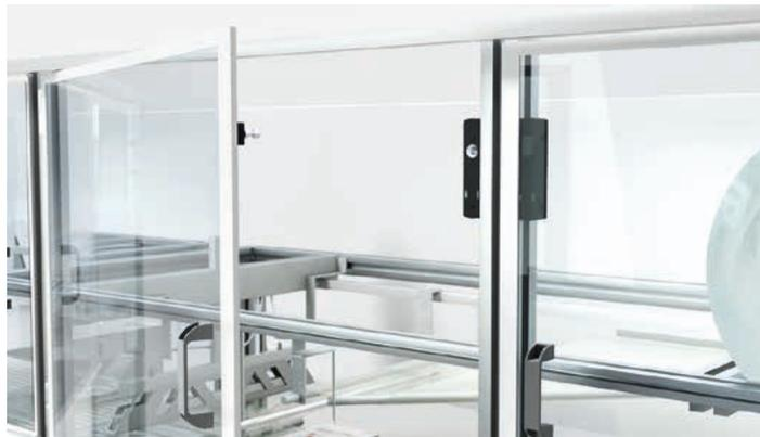
**Solution:** The L series safety switches with guard locking keep safety doors locked until the process control sends an electric release signal.
