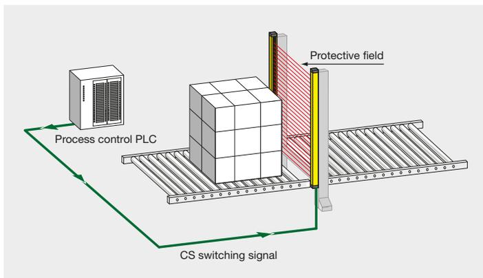
With Smart Process Gating, process control takes place in combination with the system control. A switching signal provided by the PLC and the interruption of the protective field by the transported goods are used as triggers for activating the gating function. No additional trigger sensors are required.
