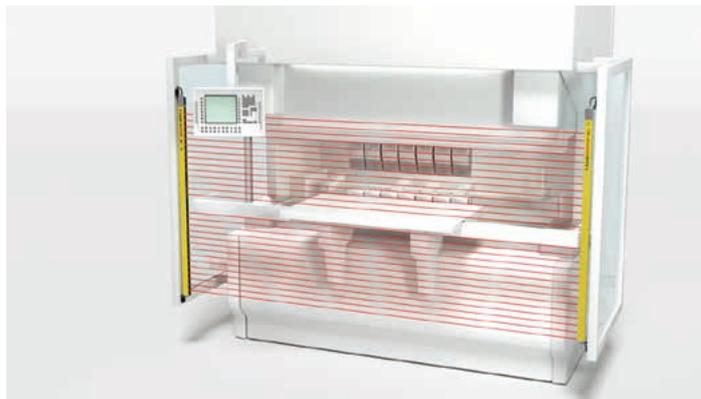
**Solution:** The MLC 530 safety light curtains have the following functions: fixed blanking, floating blanking and reduced resolution. These functions can be configured so that certain objects are permitted inside the protective field.
