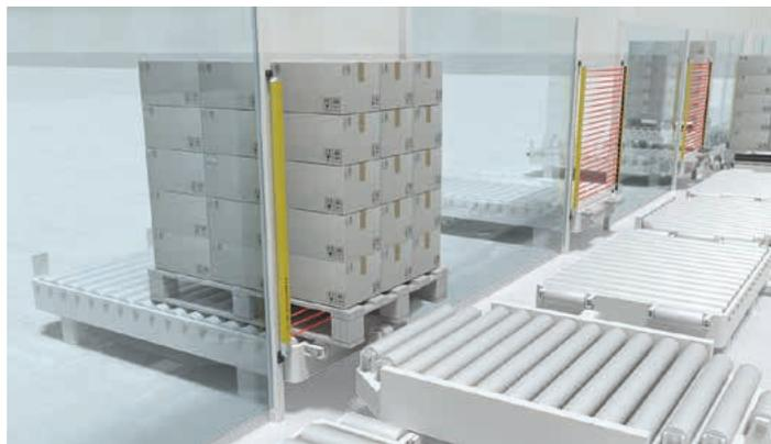
**Solution:** With Smart Process Gating, the safety sensor is bridged in combination with a control signal from the PLC. The function is integrated in the MLC 530 SPG safety light curtain. Additional muting sensors are not required and systems can be designed in a compact and space saving way.
