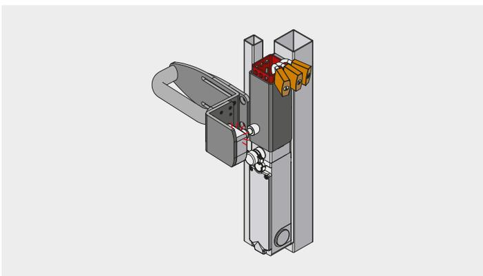
The adjustable door handle, which can be mounted on the right or left, ensures quick and easy installation of the L300 safety locking device on swing doors and sliding gates. The extremely robust metal construction supports the benefits of door centering by means of the joint on the actuator. The lockout-tagout device prevents operating personnel from being locked inside the danger zone by using individual padlocks. For this purpose, the safety mechanism is pushed downward and the lock inserted.
