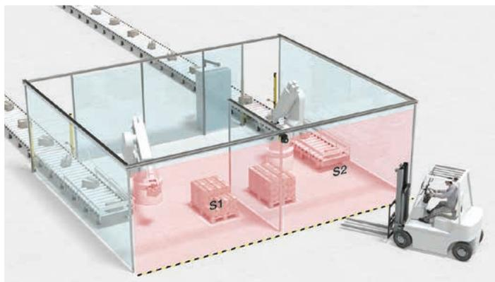
**Solution:** The RSL 400 safety laser scanner is installed above the access area and the protective field is aligned vertically. This ensures that the working area is not restricted. By using two safety functions working in parallel, one RSL 400 can monitor two stations simultaneously and independently from each other.
