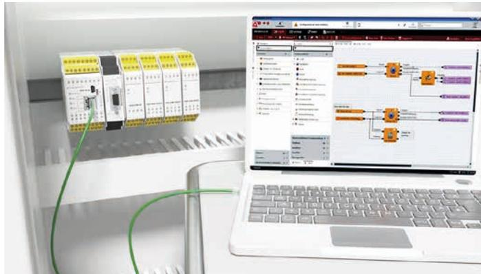
**Solution:** The basic module of the MSI 400 expandable safety control already has 24 safe inputs/outputs as well as an Ethernet interface with Industrial Ethernet protocols. The safety control can be configured quickly and efficiently using the license-free configuration software MSI.designer.
