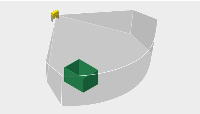
The radar technology reacts sensitively to movements. However, static objects in the monitored area do not cause the safety signal to switch off.
