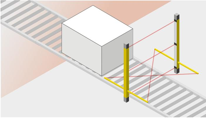
In the case of access guarding with muting function, muting sensors are used to distinguish between transported goods and persons.
