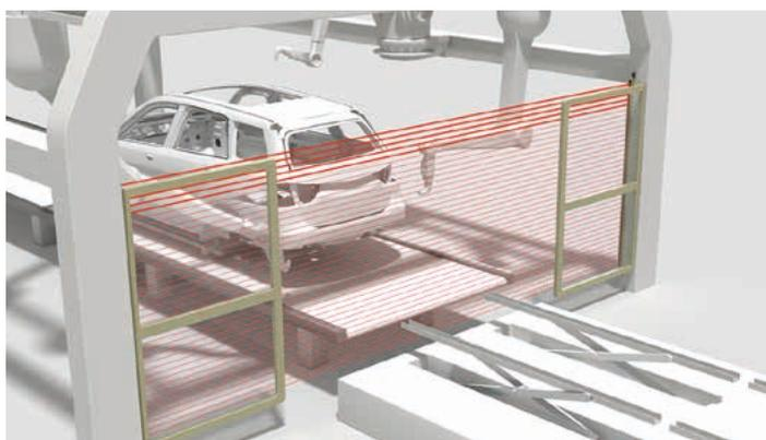
In 'Partial Gating' mode, the upper beams of the light curtain remain active during gating and can therefore be used to simultaneously monitor a second safety function. The example shows parallel monitoring of the pendulum flaps by the safety light curtain. The safety light curtain continues to monitor the closed state of the flaps also during gating. The otherwise usual safety switches for monitoring the flaps are no longer required.
