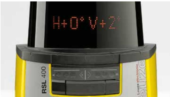
The large characters on the integrated display are easily visible even from a distance. Various functions and messages are thereby always in view.
