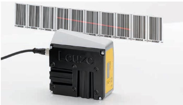
The FBPS 600i works particularly reliable. Each scanning operation reads several codes from which the software determines highly precise position values. The diagonal path of the scanning beam and the movement of the device mean that each code is scanned at different points. This prevents reading errors caused by local soiling or damage.
