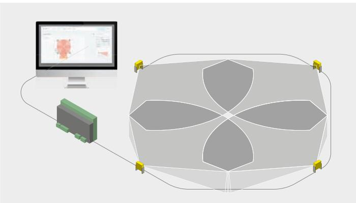
To guard large areas, up to 6 sensors can be combined in one application using a control unit. The system parameters are set using the easy-to-use configuration software.
