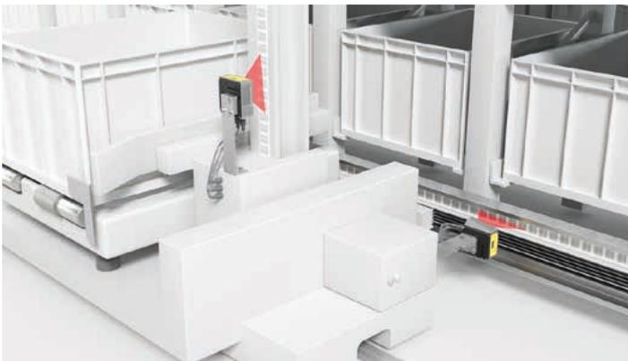
The FBPS 600i is ideal for position detection in applications involving fast movements, e.g. for use on high-bay storage devices. For this purpose, the FBPS 600i has an extremely short error reaction time of just 10 ms. This enables the optimization of speed curves and handling performance.
