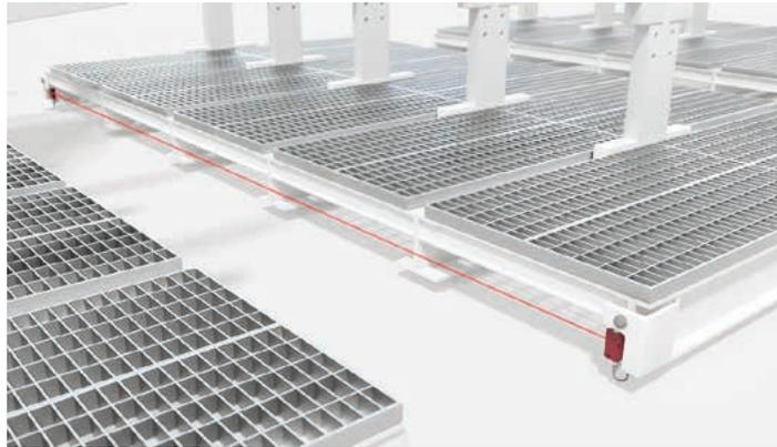
**Solution:** The SLS 46C single light beam safety devices monitor the foot space over a length of up to 70 m. They are available as a type 4 variant and as a particularly easy-to-align type 2 variant. The use of models with red light and infrared light prevents mutual interference between the shelf rows.
