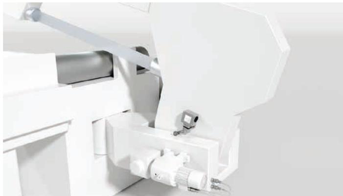
**Solution:** The S300 position switch monitors when the final position is reached. Variants with plunger and various actuators make the device suitable for universal use. With its forced normally closed contacts, the S300 can also be directly integrated into the safety circuit.
