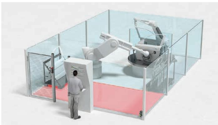
**Solution:** The RSL 400 safety laser scanner with its configurable protective field monitors the presence of persons. The LBK 3D safety radar system is used under harsh ambient conditions and also allows the presence of static objects in the monitored area.
