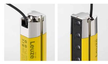
The ELC100s are easily and flexibly integrated into the machine design. The specially designed housing enables flexible cable routing in all directions. The cable is always optimally routed into the interior of the machine and protected at the same time. The protective field extends in both directions to the edge of the housing. This allows the units to be mounted flush against boundaries without creating blind zones. No additional safe-guarding measures are required.
