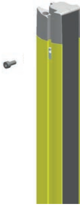
Fig. 5.6: Mounting via sliding blocks
