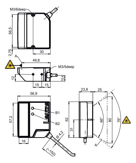
Α Laser beam Decode LED В1 B2 Status LED
