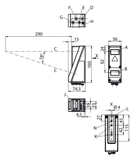
Transmitter Receiver Optical axis
