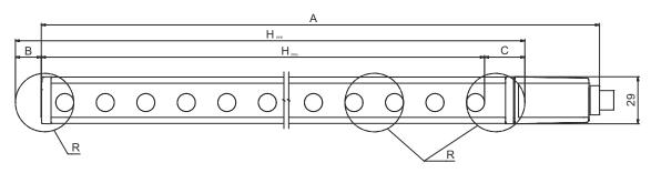
$H_{\mathsf{PFE}}$  Effective protective field height = 1062 mm H<sub>PFN</sub> Nominal protective field height = 1050 mm
