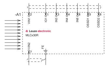
VIN1 = +24 V, VIN2 = 0 V: transmission channel C1 VIN1 = 0 V, VIN2 = +24 V: transmission channel C2
