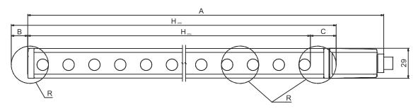
$H_{\text{PFE}}$  Effective protective field height = 1812 mm  $H_{\text{PFN}}$  Nominal protective field height = 1800 mm
