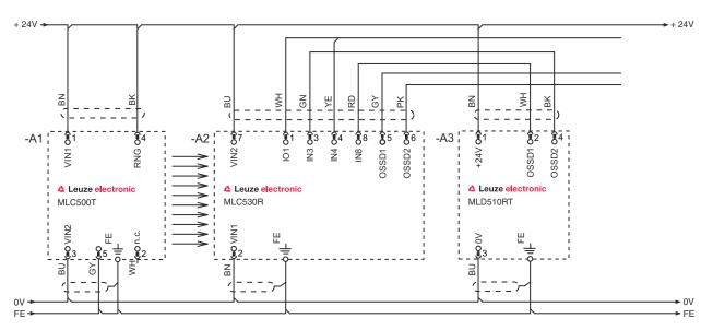
Operating mode 3: circuit diagram example of a linked, contact-based position switch for monitoring of the blanked object and a changeover switch for switching between function groups FG1 and FG2
