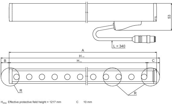
$H_{PFE}$  Effective protective field height = 1217 mm  $H_{PFN}$  Nominal protective field height = 1200 mm
