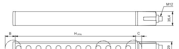
$H_{\mathsf{PFE}}$  Effective protective field height = 1662 mm  $H_{\mathrm{PFN}}$  Nominal protective field height = 1650 mm
