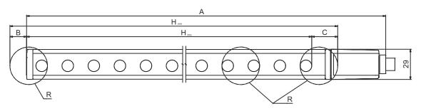
$H_{\mathsf{PFE}}$  Effective protective field height = 790 mm H<sub>PFN</sub> Nominal protective field height = 750 mm
