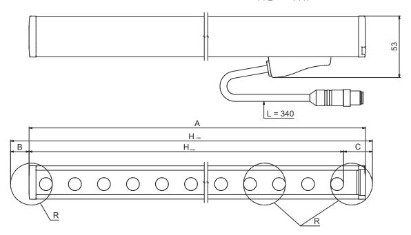
$H_{\mathsf{PFE}}$  Effective protective field height = 640 mm  $H_{\mathrm{PFN}}$  Nominal protective field height = 600 mm
